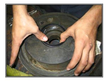
Apply grease to the plug seal (5) in the adjusting nut (12).
