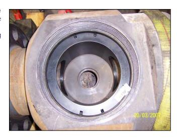
Apply a thin film of lubricant to the recess in the adjusting nut (12) and install the plug seal (5) with the metal back towards the recess facing away from the pressure.
