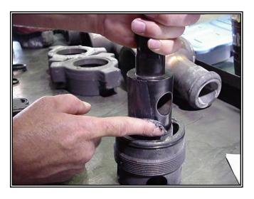
Check the surface finish of the inserts (12) making sure they do not have any scratches, dings, nicks or sharp edges that could affect the sealing area.
