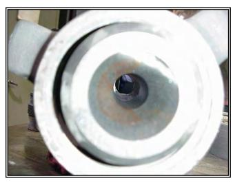
$\circ\$  Grease the counter bore of the valve body female end and press the resilient
