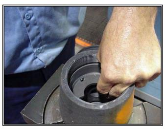
o Apply a thin film of lubricant to the recess in the **valve body (8)** and install the **plug seal (9)** with the metal back towards the recess facing away from the pressure.
