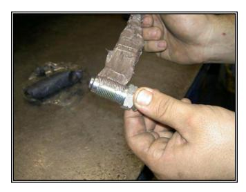
o Remove excess grease from valve bore.
