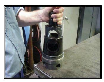
o Place the insert o-rings (11) in to the grooves on the UNIsert™ (12) and pack with grease to retain the rings and thoroughly grease the sealing surfaces.
