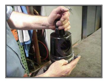
Secure the plug (10) to the adjusting nut (14) with the plug bolt (1) and two washers (2 & 3).
