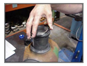
o Then place wing nut (17) on male end and install the nut retainer set (18) (if required).
