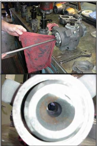
Inspect plug alignment and adjust as necessary with adjusting nut (14).
