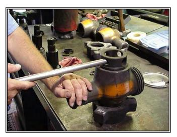
Apply thread compound (Never Seez) to the threads on the SafeTap™ grease fitting (7). Install grease fitting and torque to 80 ft-lbs.
