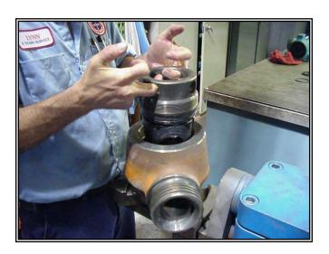
o Screw in the adjusting nut until proper alignment is obtained between the valve bore, the UNIsert™ and plug. Do not tighten beyond proper alignment as actuating an over tightened valve could damage internal parts. If sight through the bore is not possible, then screw in the adjusting nut until ½ or no thread is visible.
