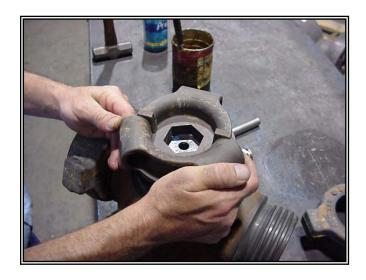
o Secure handle adapter (4) with the plug bolt (1) and washers (2 & 3).
