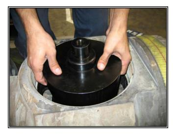
c Check the surface finish of the **inserts (7)** making sure they do not have any scratches, dings, nicks or sharp edges that could affect the sealing area. See **8.2 SANDING TIPS** for repair.
