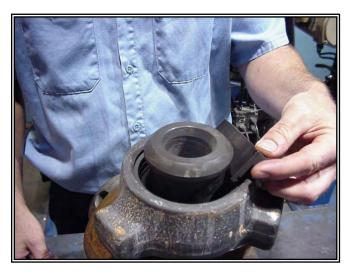
Secure the retainers with spiral retainer ring (if required)
