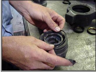
Check the roll pins (15 & 16) in the valve body by gently sliding a set of inserts (12) into the valve. The inserts (12) should move freely up and down the length of the roll pin slots without interference.
