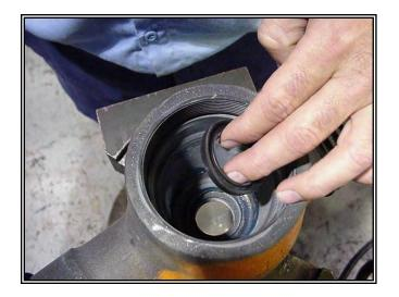
Apply a thin film of lubricant to the recess in the adjusting nut (14) and install the plug seal (9) with the metal back towards the recess facing away from the pressure.
