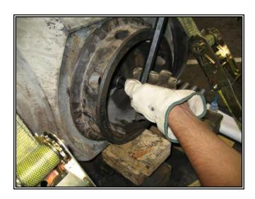
Apply thread compound (Never Seez) to the threads on the SafeTap™ grease fitting (2). Install grease fitting and torque to 80 ftlbs.
