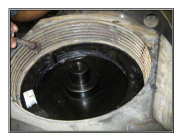
Grease the seal ring (10) groove and insert the o ring
