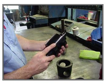
o Check the surface finish of the **UNIsert™** (12) making sure it does not have any scratches, dings, nicks or sharp edges that could also affect the sealing area. See <u>8.2</u> SANDING TIPS for repair.
