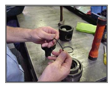
Pack the adjusting nut (14) plug seal (9) with valve grease.
