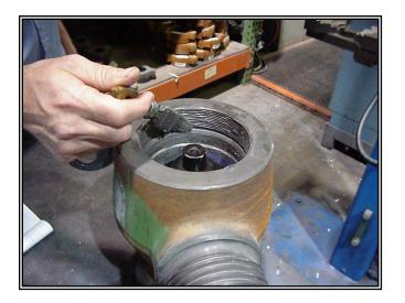
Support the valve so that the **plug (10)** hex can pass through unobstructed.
