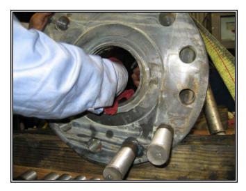
Inspect plug alignment and adjust as necessary with adjusting nut (12).
