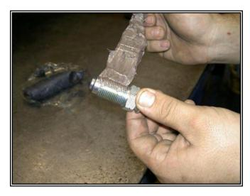
o Remove excess grease from valve bore.
