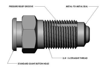
• The metal-to-metal seal and the pressure relief slot of the **SafeTap™** grease fitting also allow a means to safely bleed any residual internal pressure.
