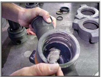
Install the plug (10), inserts (12) and adjusting nut (14) assembly into the valve body.
