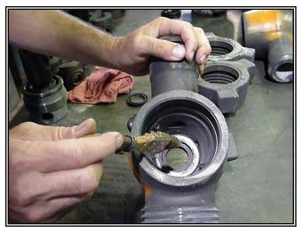
Apply thread compound (Never-Seez) to the adjusting nut threads and adjusting nut sealing surfaces.
