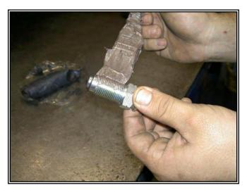
Install SafeTap<sup>™</sup> grease fitting (7) and torque to 80 ft-lbs.
