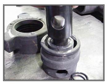
Apply a thin film of grease to the entire O.D. of the plug (10).
