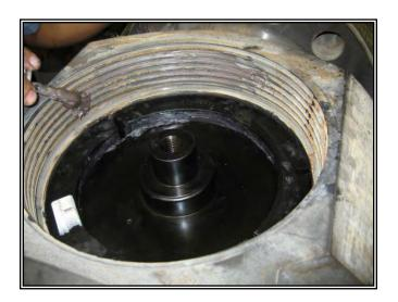
Grease the seal ring (10) groove and insert the o ring (9) over it.
