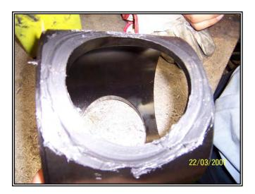
Apply a thin film of grease to the entire I.D. of the insert (7).
