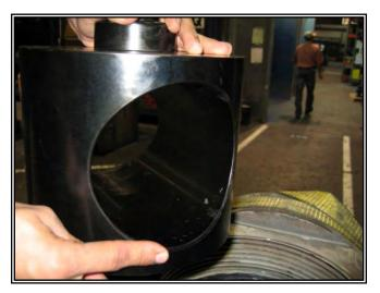
Support the valve so that the plug hex can pass through unobstructed.
