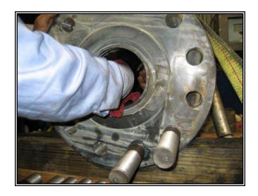
Inspect plug alignment and adjust as necessary with adjusting nut (12).
