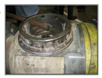
Apply thread compound (Never Seez) grease to the plug bolt (14) threads and tighten it with the allen wrench on the adjusting nut side of the plug (6).
