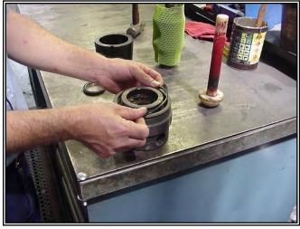
Check the roll pins (15 & 16) in the valve body by gently sliding a UNIsert™ (12) into the valve. The UNIsert™ (12) should move freely up and down the length of the roll pin slots without interference.
