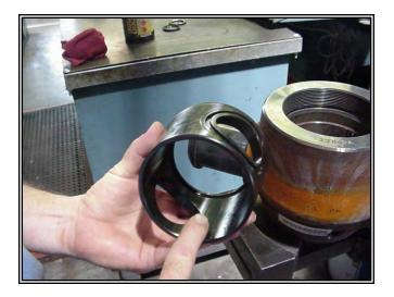
Inspect the adjusting nut o-ring (13) for any possible non-conformity.
