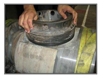
o After inspection remove the adjusting nut and check the roll pins (15 & 16) in the valve body by gently sliding a set of inserts (7) into the valve. The inserts (7) should move freely up and down the length of the roll pin slots without interference.
