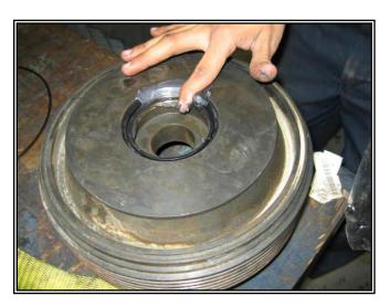
Grease the sealing groove and install the adjusting nut o ring (11) in the groove.
