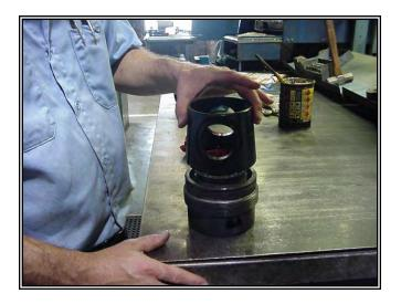
o Apply a thin film of grease to the entire O.D. of the **plug (10)**.
