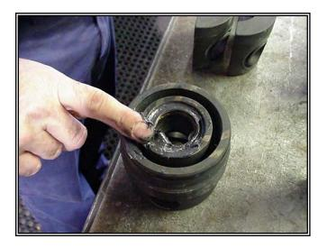
Install the lower end of the plug (10) (opposite the hex) in the adjusting nut (14) and push down until the plug shoulders on the adjusting nut.
