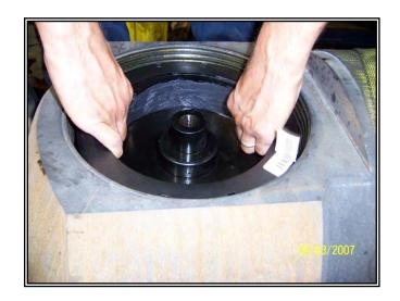
Apply thread compound (Never-Seez) to the adjusting nut threads and adjusting nut sealing surfaces.
