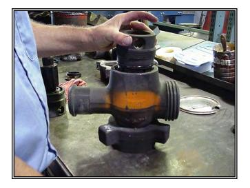
Tighten the adjusting nut (14) until snug and back off ¼ turn from snug position.
