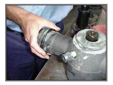
o Then place wing nut (17) on male end and install the nut retainer set (18) (if required).
