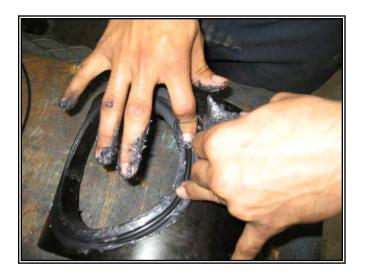
o Make sure the entire sealing surface is thoroughly greased.
