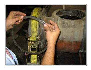
o Place the **seal ring (10)** on the top of the **insert (7)**.
