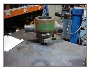
Install the plug (10), UNIsert™ (12) and adjusting nut (14) assembly into the valve body.
