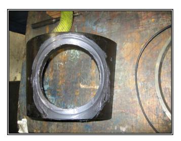
Apply a thin film of grease to the entire I.D. of the insert set (7).
