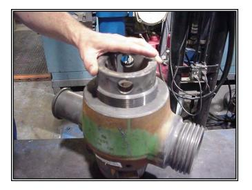
Apply thread compound (never Seez) to the threads on the SafeTap™ grease fitting (7).
