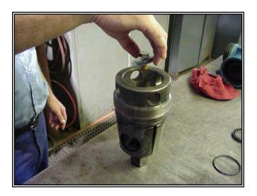
o Lubricate the valve pocket with valve grease.
