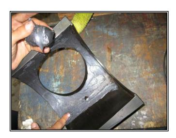
o Place the **inserts (7)** around the **plug (6)** in the valve body making sure it slides into the roll pins.
