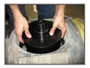
Check the surface finish of the insert (7) making sure they do not have any scratches, dings, nicks or sharp edges that could affect the sealing area.
