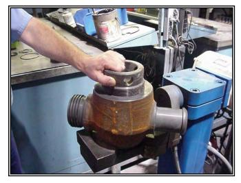
After inspection, remove the adjusting nut (14), grease the sealing groove and install the adjusting nut o ring (13) in the groove.
