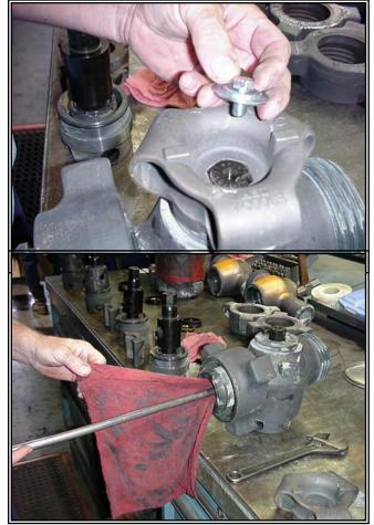
o Remove excess grease from valve bore.
